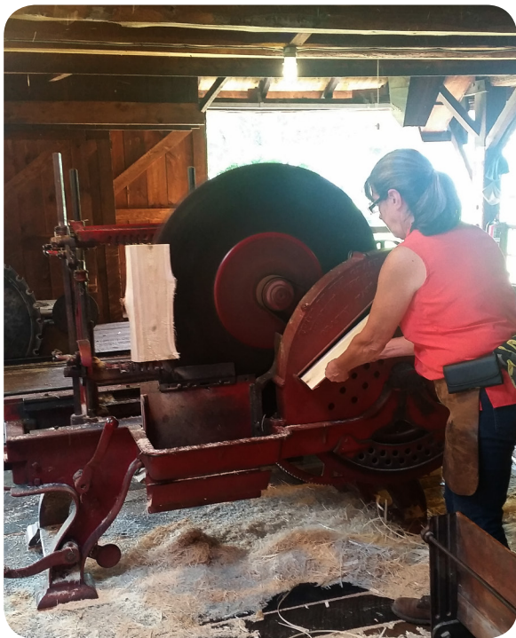
Dawn Raughdibaugh planing the edges of a shingle using the Chase Shingle Mill.
