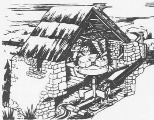
An early Greek style waterwheel powering a gristmill. Illustration from Stronger than a Hundred Men by Terry S. Reynolds.
