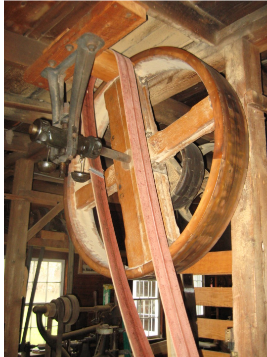
A 40-inch diameter pulley manufactured by the Ohio Valley Pulley Works, Maysville, Kentucky. This pulley drives the C.B. Rogers & Co. 16-inch jointer located in the box room.
